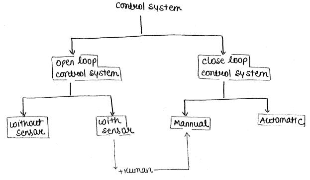
differences between open loop and close loop system:
