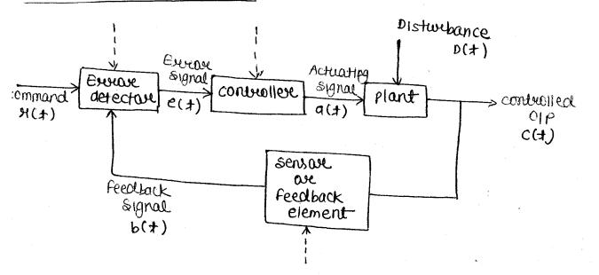
$C(t) = C_{H}(t) + C_{D}(t)$  [Unear combination because H(t) & D(t)] both are independent to each other]
